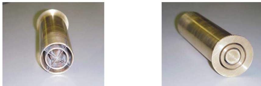
Fig. 5. The inlet and the exit of the model for water tunnel. The dimensions are shown in Fig. 6, the diameters are half of those given in Table 1.
